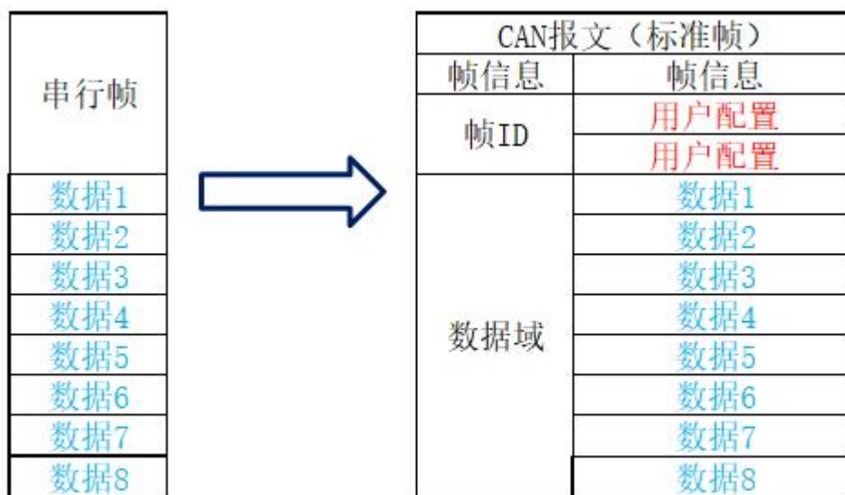
Figure 4.5 Frames in UART converts to CAN message(Transparent band information conversion)
