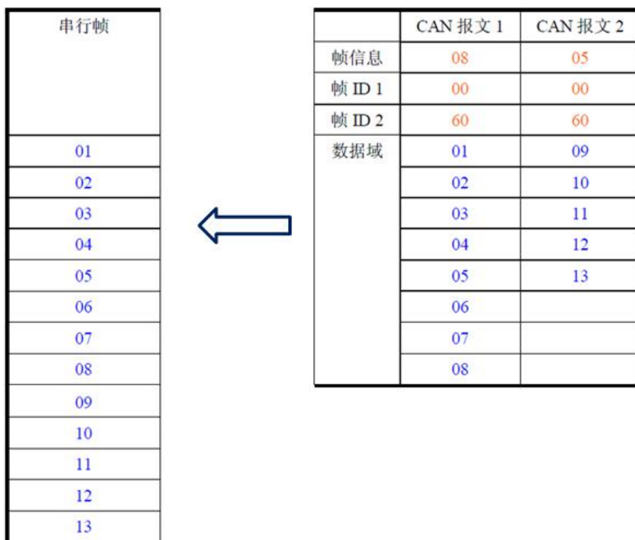
Figure 4.4 CAN message converts to frames in UART (Transparent conversion)
