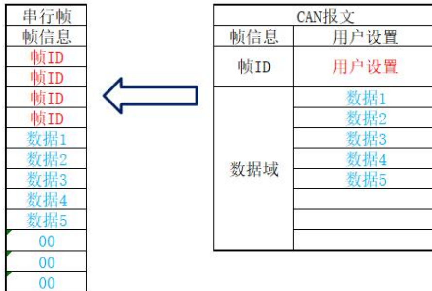
Figure 4.7 CAN message converts to frames in UART (Transparent band information conversion)
