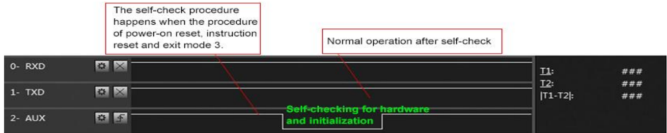
Timing Sequence Diagram of AUX when self-check
