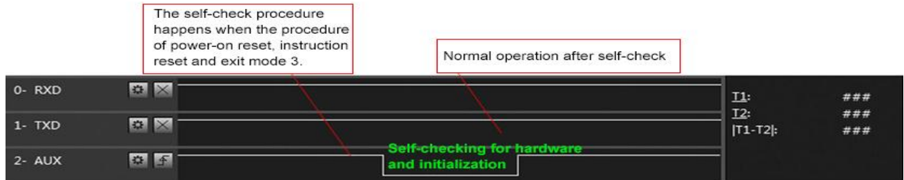
Timing Sequence Diagram of AUX when self-check
