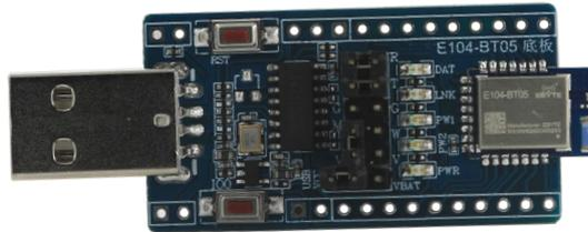
The test backplane of E104-BT05-TB adopts USB interface, which can be used to quickly test the features and functions related to E104-BT05 Bluetooth.
