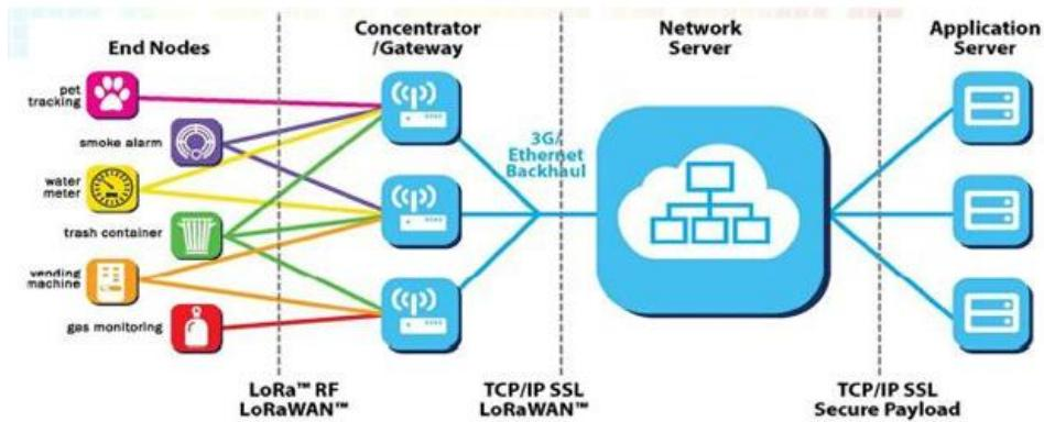
The complete LoraWan network system is composed of nodes, gateways, Lora Network Server and application servers. The nodes are generally designed by LORA chips; The gateway is designed by SX1301 provided by semtech; Lora NetWork Server now has an open source loraserver or a commercial TTN (The ThingsNetwork) in the industry, which users can build by themselves; The application server is designed and developed by users and is mainly used to exchange application data with Lora NetWork Server.
