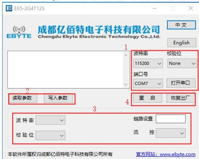
Figure 4-6 Configuration software interface
