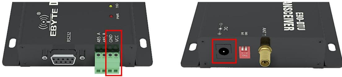
2、 Using USB-(RS232) converter or USB-RS(485) converter or other way to link computer and DTU.
